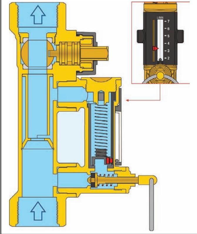
This valve, which can be mounted in any position, also allows adjustment of flow rate by turning the stem located above the flow meter.
