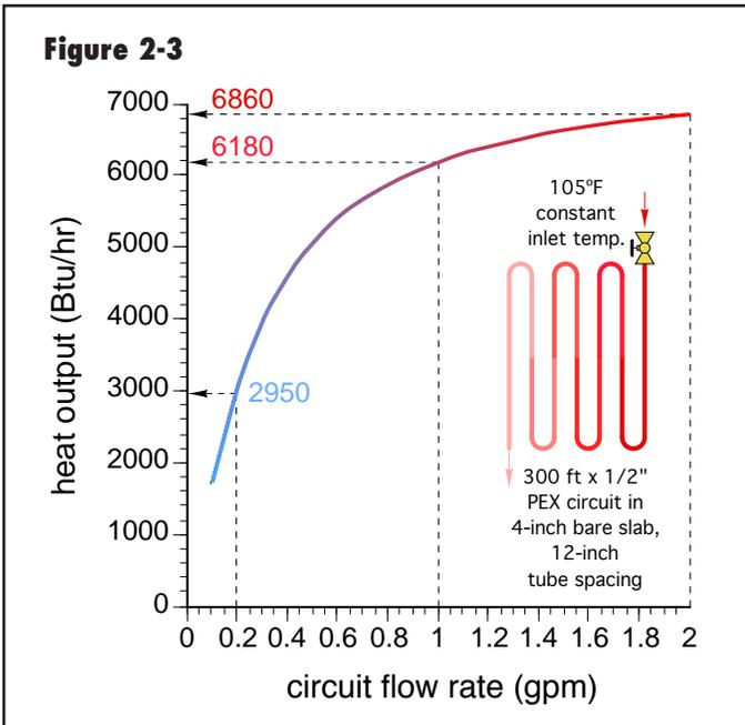
This floor heating circuit's maximum heat output of 6,860 Btu/hr occurs at the maximum flow rate shown, (2.0 gpm). Decreasing the circuit's flow rate by 50% to 1.0 gpm decreases its heat output to 6,180 Btu/hr, a drop of only about 10%. Reducing the flow rate to 10% of the maximum value (0.2 gpm) still allows the circuit to release 2,950 Btu/hr, about 43% of its maximum output.
