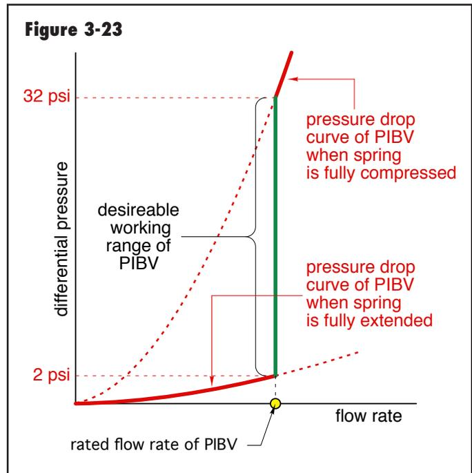
With a PIBV in each crossover, the flow rates through each *active* crossover remains at its design value, regardless of the flow status in other crossovers. However, this desirable condition is contingent upon keeping the differential pressure across the PIBV between its lower and upper threshold values. This condition is vitally important to proper application of such valves, and will be discussed further in section 5.
