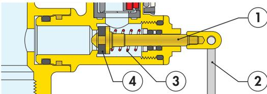
The operating ring (2) material has low thermal conductivity to avoid burns if the flow meter is opened while hot fluid is passing through the valve.
