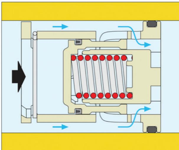
The unique polymer cartridges used in all Caleffi PIBVs are specifically designed for low flow noise.
