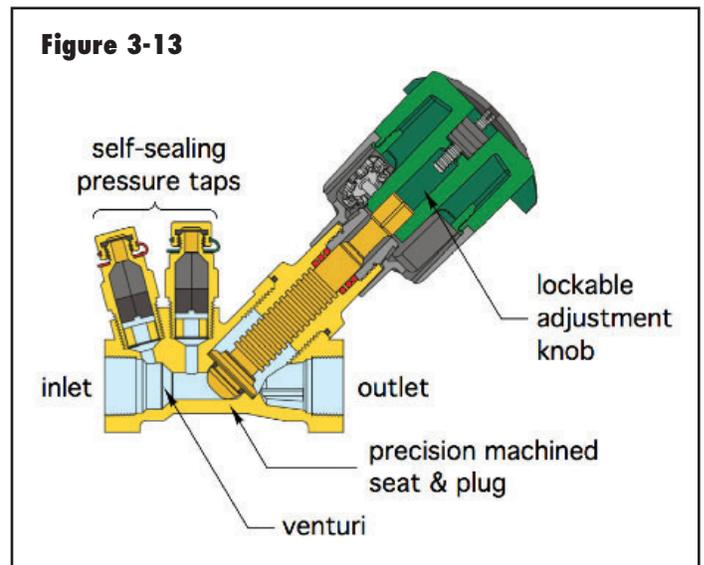
All valves with pressure taps require the use of a measuring instrument to read the differential pressure that infers the flow rate through them. An example of such a device is shown in figure 3-14.
