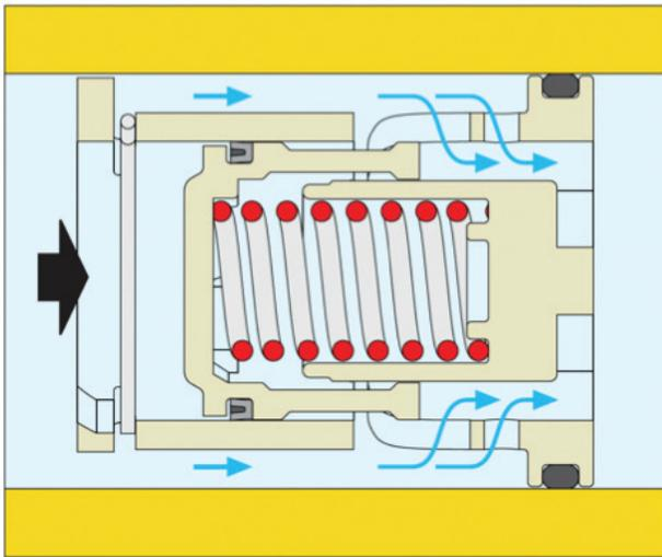
This ability to adjust flow through the tapered orifice remains in effect until the differential pressure across the valve exceeds an upper threshold limit of 14, 32, 34, or 35 psi (depending on valve model). Such high differential pressure is relatively uncommon in most well-designed hydronic systems that include some means of differential pressure control.
