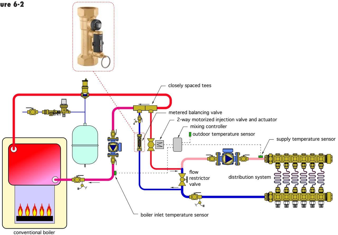
For optimal performance, the injection control valve and the flow-restrictor valve need to be properly selected and adjusted. The following selection and adjustment procedure applies to both 2-way thermostatic and 2-way motorized injection control valves.
