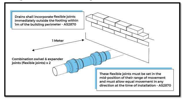
Articulation detail – Eternal to slab, for soil classifications H1, H2 and E
