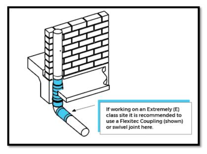
Storm Water Detail – Downpipe through slab for soil classifications H1, H2 and E
