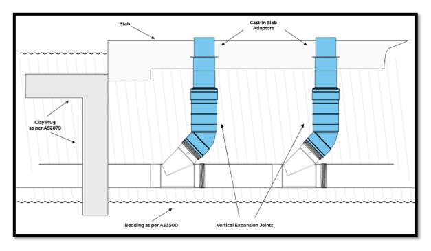
Articulation to be provided under the slab for soil classifications H1, H2 and E
