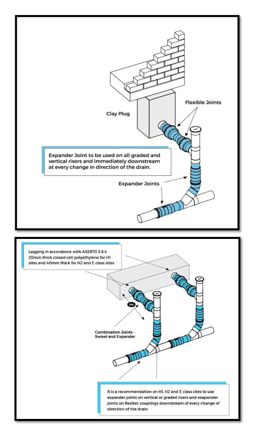
Articulation Provided at changes of direction and immediately downstream at every change of direction – Pipes to be lagged where passing through concrete for soil classifications H1, H2 and E
